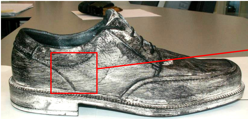
Picture 19: Result of the 0.4mm nylon brush
